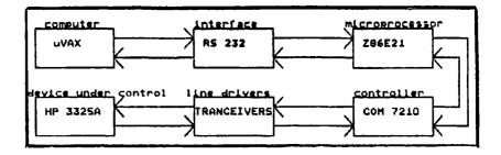
The card controls and communicates any compatible instrument with the standard. It implements the full range of talker, listener, controller and remote programming functions.
